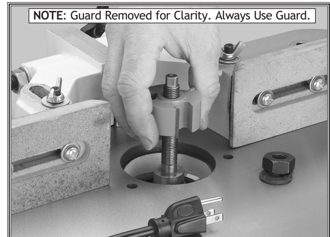
Figure 6. Unplug the shaper whenever making adjustments or changing cutters.
